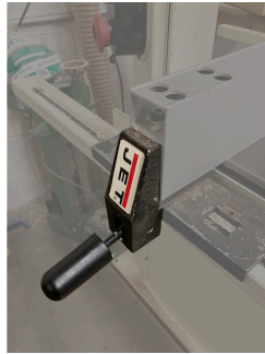
Figure 7: Lift the fence release lever before adjusting the fence.
