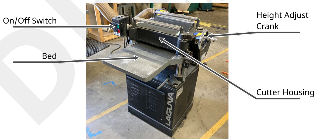
Figure 8: Front quarter view of the planer.
