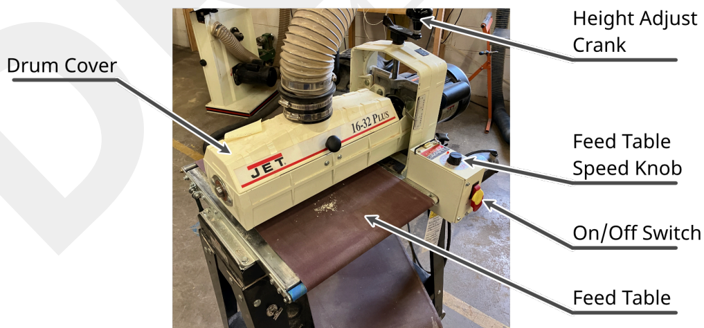
Figure 9: Full view of the drum sander.
