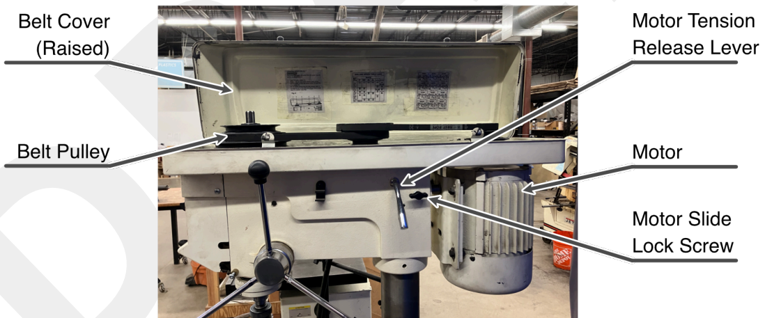
Figure 4: Annotated view of the belt drive system.
