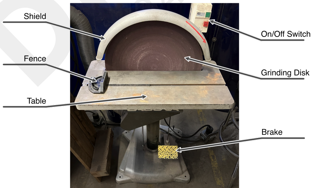
Figure 9: Front view of the disk grinder.
