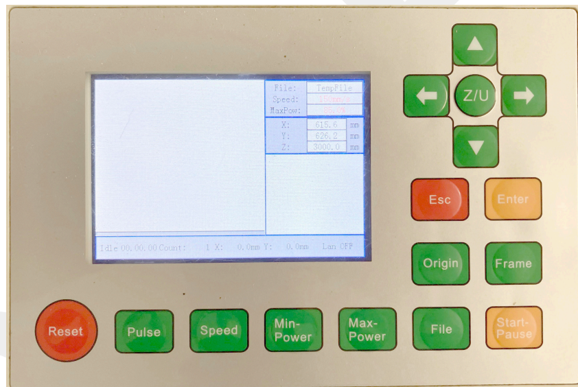
Figure 2: The control panel for the large format laser in the default view.
