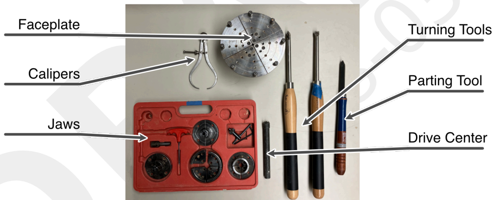
Figure 3: Contents of the lathe accessory kit.
